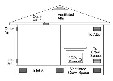
Figure 3 - Ventilation Air from Outdoors
